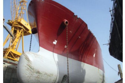
Performance on a LNG tanker after 30 months in-service. Excellent performance with minimal slime level.
